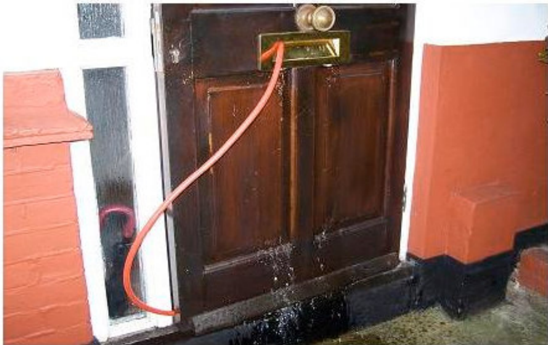
Rubber water hose was used for introducing water jet into the letter box protected by IdealGuard™ . On the bottom photo one can see water flowing out of the letter box and streaming down the door surface to the ground.
