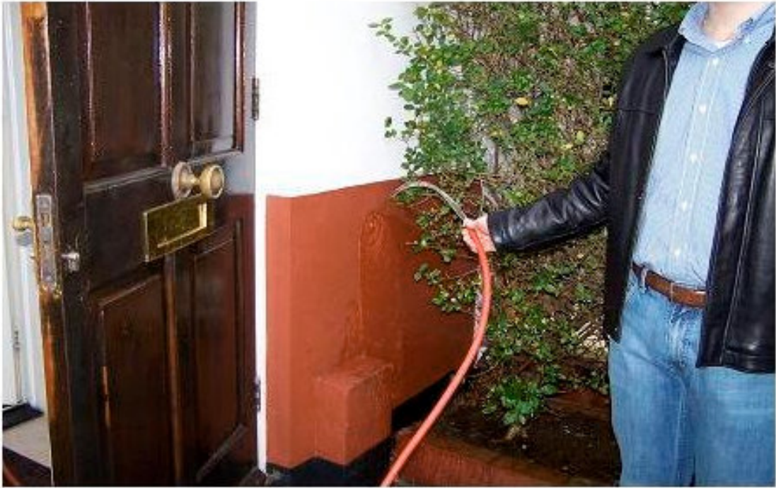
Rubber water hose was used for introducing water jet into the letter box protected by IdealGuard™ . On the bottom photo one can see water flowing out of the letter box and streaming down the door surface to the ground.
