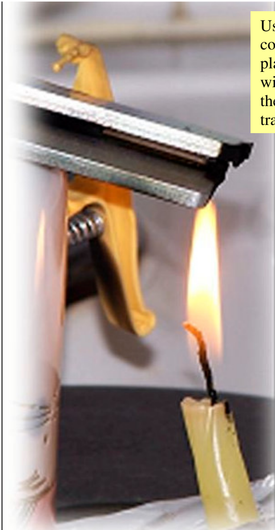
The Seal sample was glued to a metal plate before the test
